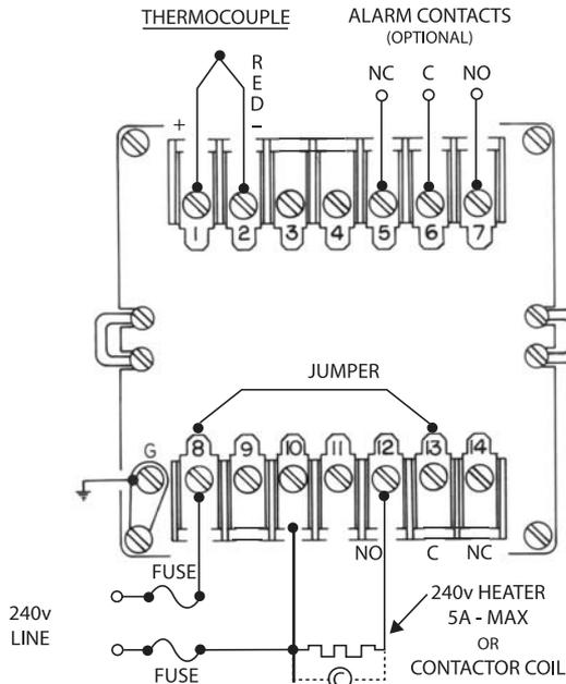
Figure 2a: Typical 240 Vac for -B & -T Output
