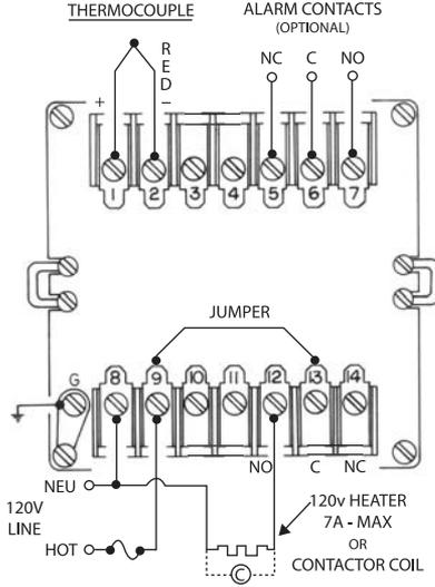
Figure 2b: Typical 120 Vac for -B & -T Output
