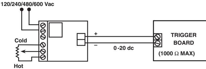
Figure 7. Wiring diagram for thermostatic control (Option H required).
