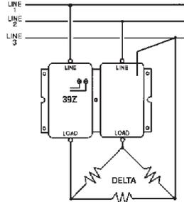
Figure 4b. Wiring scheme for Series 39Z.
