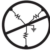
On Wye connected loads, do not connect the center terminal to the line or to the ground.
