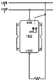
Figure 4a. Wiring scheme for Series 19Z.
