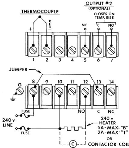
Figure 2: Typical 120 Vac for -B & -T Output
