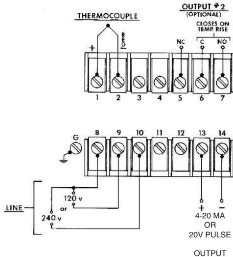
Figure 3: Typical 120/240 Vac for -F and -S Output
