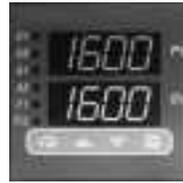
Experienced users, already familiar with the Series 16C, and using the controller with PID outputs, may follow these condensed instructions to autotune the controller and get started quickly once the instrument is properly mounted and wired, and the Security Level is set to **Level 4**. Once setup is complete, we recommend changing the Security Level back to the most restrictive level suitable for your application.
